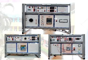
Static over current Relay Trainer, Static over voltage Relay Trainer and Static Negative Sequence Relay Trainer are available in Switchgear and protection lab
