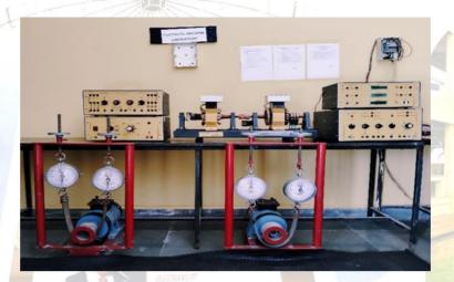
**Electrical** Machine **Open** Lab Set (DYNALOG): The system is a component kit that should allow to assemble the rotating electrical machines, both for AC/DC. Set contains Power supply unit, Electrical and speed measurement module, Load and rheostat module, adapter bracket, Locking and rotatable device, Parallel Board, Starting and Synchronization unit, Electromagnetic Break, Star-Delta starter, Pole changing Unit
