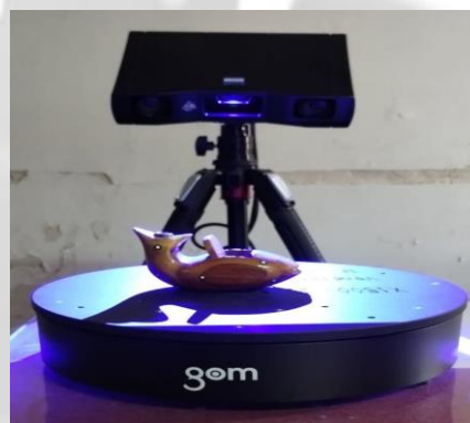
3D Scanner GOM Scan 1 System Package including GOM ROT 350 Rotary table
