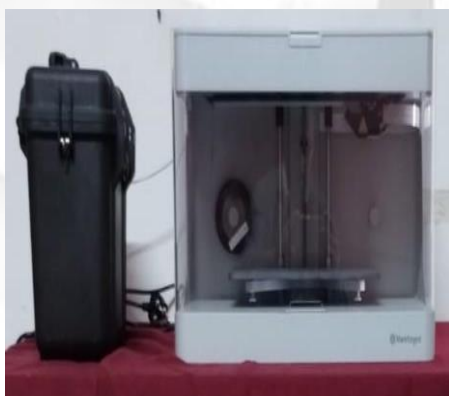
FDM based composite 3D Printer Mark Two, 2ND Generation Build volume : 320 x 132 x 154 mm (WidthxDepthxHeight)
