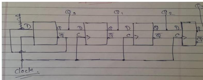
8. Complete the timing diagram for this circuit, showing propagation delays for all Flip-flops (delay time much less than the width of the clock pulse), assuming all Q outputs begin in the low state.
