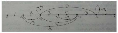
Q.10 Using mason gain formula find the transfer function  $\frac{c}{R}$  for the signal flow graph [L3,CO1] 10M shown in figure.
