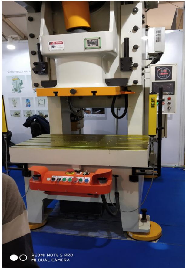
Cam follower operated Punch Press Machine
