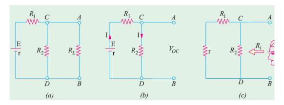
Suppose, it is required to find current flowing through load resistance RL, as shown in Fig. (a).
