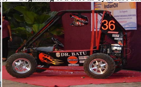
All terrain vehicle made by students of SAE Collegiate Club for SAE BAJA Competition
