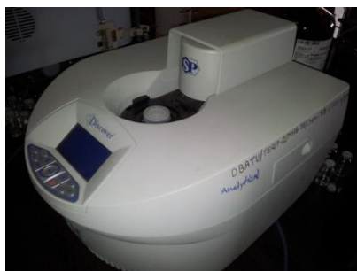
FOCUSED MICROWAVE FOR SYNTHESIS
